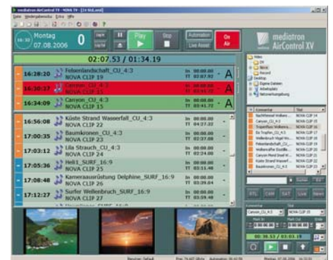
AirControl XV Playout Videosever for fully automated and live assist broadcast control
